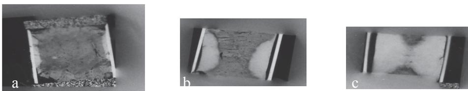
**Figure 128 :** Autoradiographs of samples in which the polymerisation of MMA was performed by heating. Samples taken at a) 15cm, b) 70cm and c) 100cm deep. The C-14 MMA intrusion was not complete; the light areas on the autoradiograph were not impregnated with MMA or the MMA had evaporated/outleached from the matrix during polymerisation.
