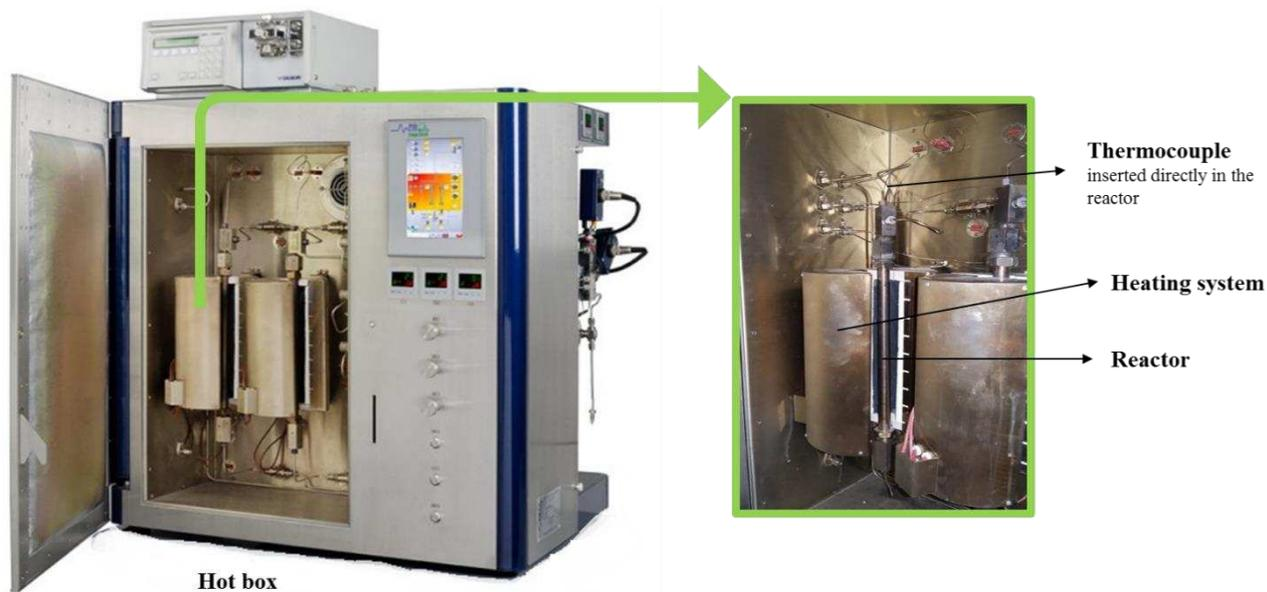
Figure II.12 Reactors and heating systems.
