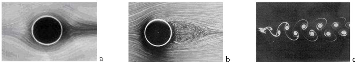
Fig 3.1 : Ecoulement derrière un cylindre (Van Dyke): (a)  $Re = 1$  (b)  $Re = 26$  (c)  $Re = 105$
