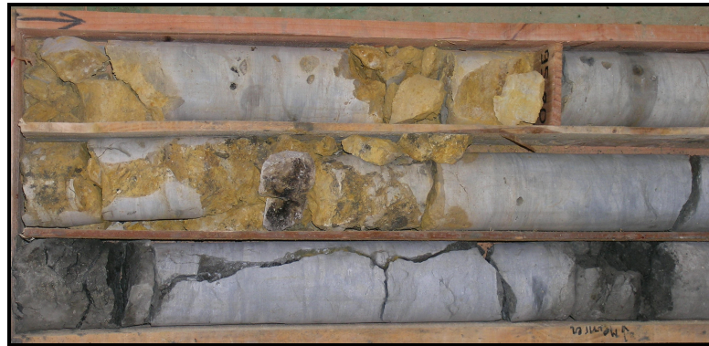
Figure 1.8: Cores from C2 well at about 97m depth: clay material is filling the upper "damaged" zone (karst residue) ; a vertical fracture is observed between two marly (dark) layers in the lower core.
