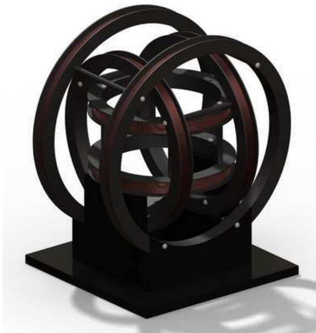
FIGURE 1.26 – Bobines de Helmholtz tri-dimensionnelles (Micro Magnetics, Inc)
